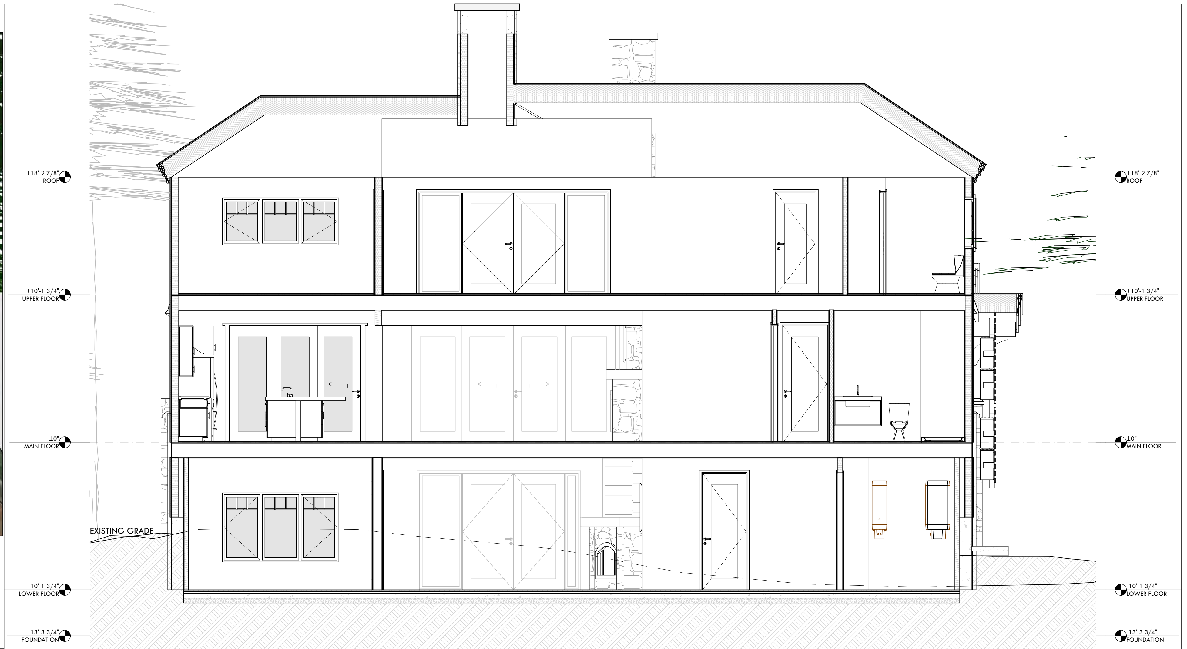
1 LONG BUILDING SECTION SCALE: 1/4" = 1'-0"
